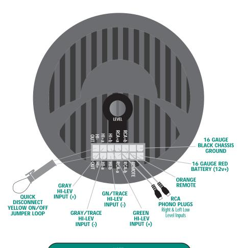
NOTE: REMOVE AUTO TURN-ON LOOP TO USE ORANGE REMOTE WIRE FOR NORMAL REMOTE TURN-ON
